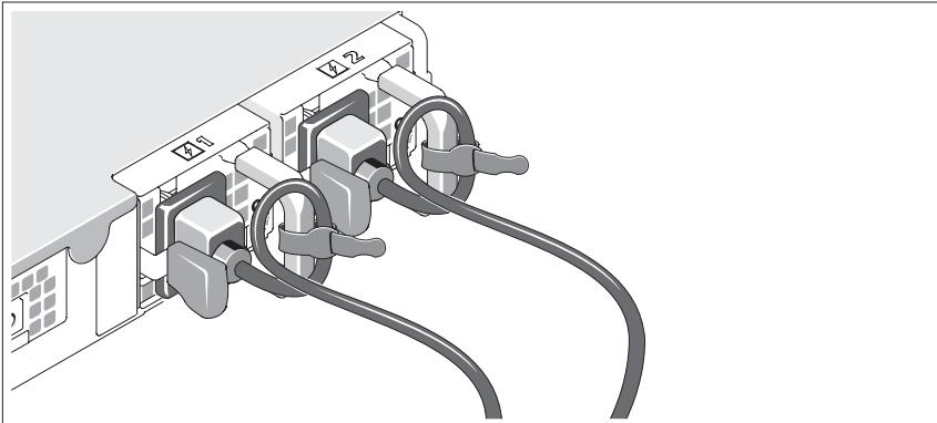
Connect the system's power cable(s) to the system (a redundant system is shown in the illustration). For redundant systems, secure the cables with the two Velcro straps that ship with your system, as shown. For non-redundant systems, attach the power cord retention bracket that ships with your system.
